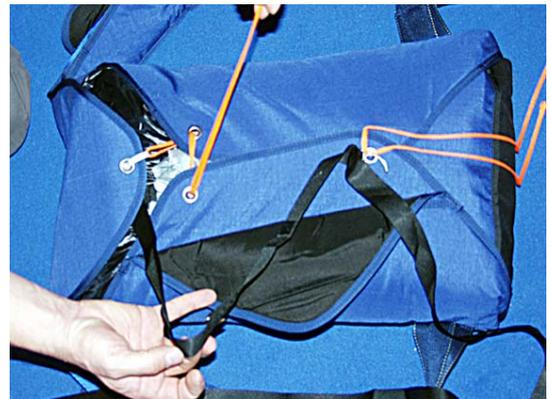
Fix the small velcrosnap on the bridle between the two pins. It is important to give extra length to allow the first pin to get out easily.
