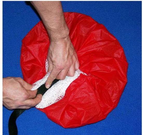
Now quarter the ZeroP fabric to keep the mesh and the bridle inside the handdeployment.
