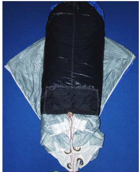
S-fold the lower part inside under the tailpocket.
